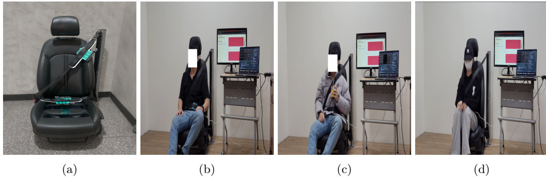
Figure 3: Illustrations show the testbed of data collection experiments: (a) Driver seat attached with belt and seat pressure sensors. Figures [(b), (c), and (d)] show participants under different postures, clothes, and gender settings.
