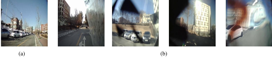
Fig. 1. The dataset sample. (a) A normal frame. (b) The failure frames of different occlusion rates from 30% to 100%.
