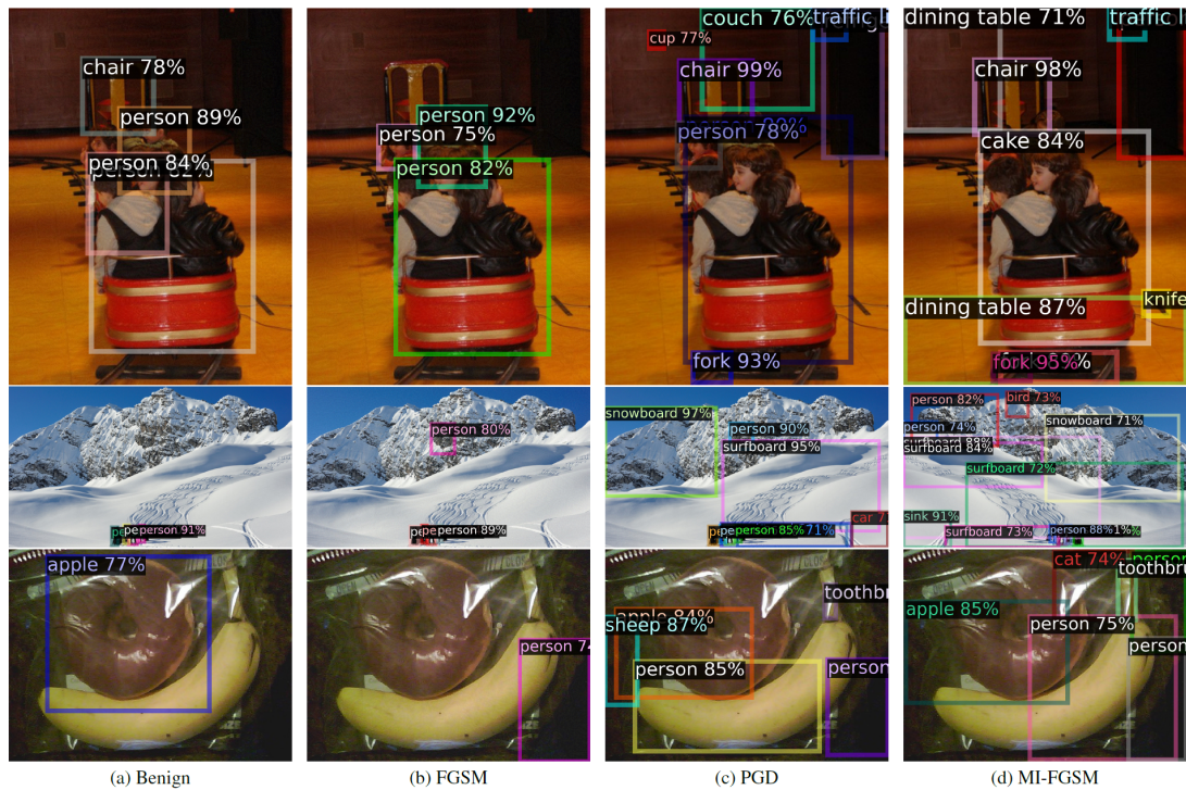
Fig. 2. Illustration of detection in adversarial examples. Benign images are shown in the first column, and three other attack methods are shown in the second to the fourth column. We only visualize the adversarial examples from the Unbiased Teacher since STAC shows a similar pattern.
