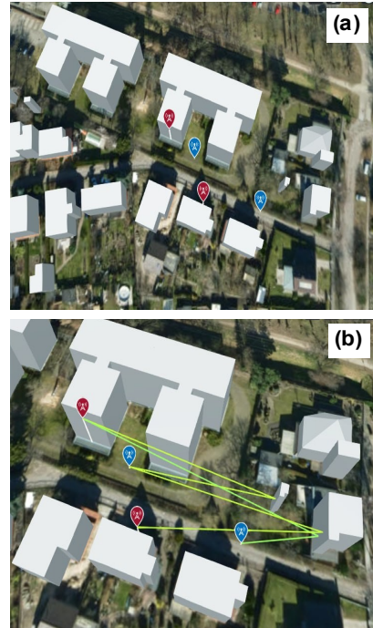
Fig. 1. (a) The city layout model. (b) The antennas placement in the model city [8].
