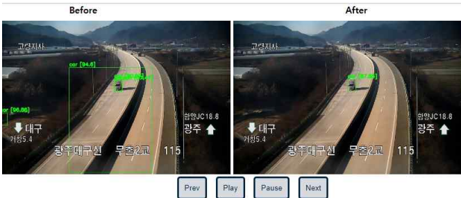
Fig. 6. Before and after of the optimization of the local customized object detector
