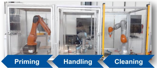
Fig. 5 Robot-based glass pane completion use case
